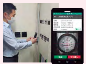
Meter reading using AI image analysis
